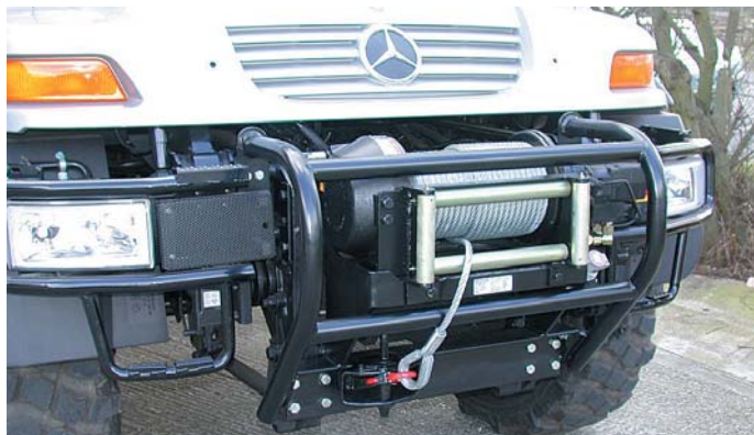
Similar to the RPH 53.3 shown here, the RPH 42.2 can be front bumper mounted on high GVW 4x4 utility vehicles.
